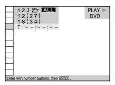
Input the time code using the number buttons, then press ENTER.
